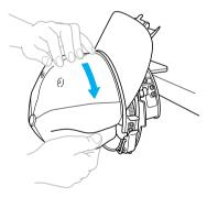
Use the clips to secure the cap.
